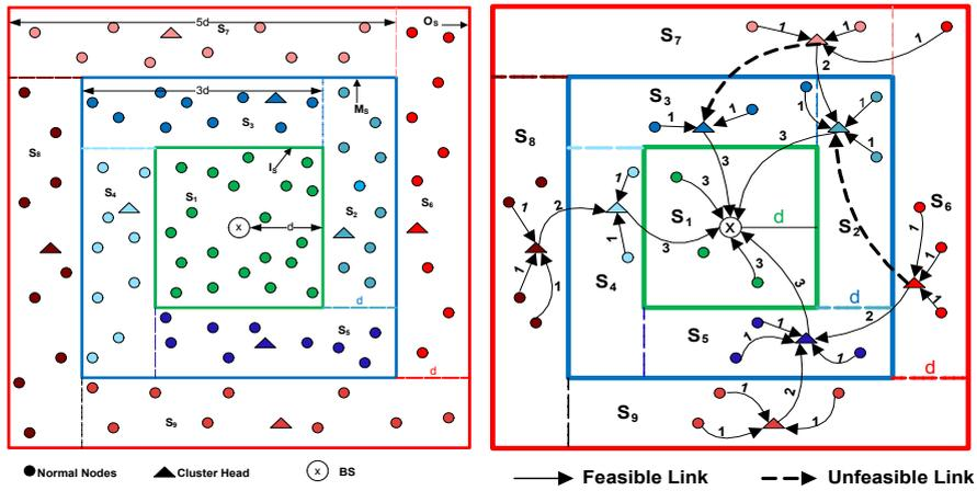
Fig. 1. (a) Deployment of nodes; (b) Communication Architecture.
